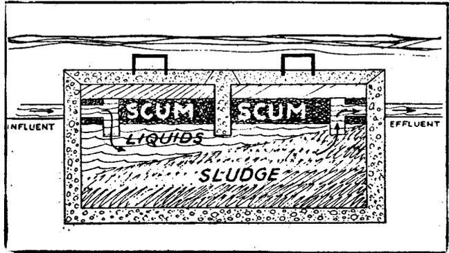
Sketch Number Two shows a tank where sludge accumulation has reached a point where solids are being flushed into the drain field. The solids will soon clog the drain field and the toilet will be slow to flush or overflow upon flushing.
