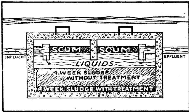
Sketch Number Four is used to show the difference in sludge accumulation with and without treatment in an already operating tank. It should be noted here, as it is important upon the effect in the drain field, that the enzymes are water soluble and therefore are gradually flushed into the drain field where further benefits are derived.
