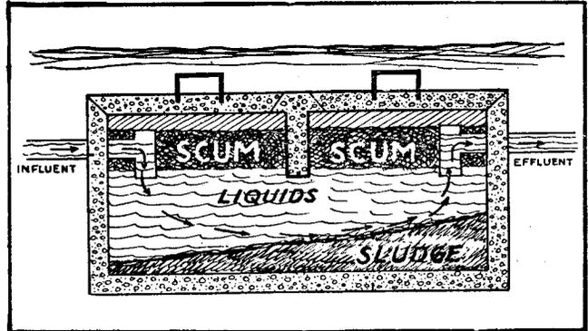
Sketch Number One shows a normally operating septic tank under proper design prior to accumulation of digested sludge in the amount that would require cleaning.
