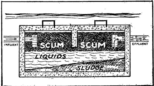
Sketch Number Three shows a heavy scum layer, often caused by the introduction of large quantities of cooking fats, or yeast. In this case, either regular treatment with ACTI-ZYME or the installation of an efficient grease trap in the line is required. If a grease trap is installed, regular cleaning of the trap must be maintained.
